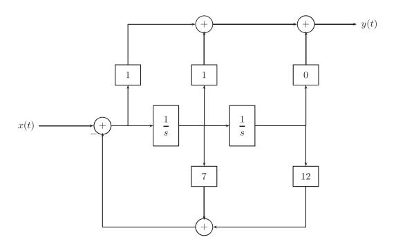
From this representation of the system, the numbers in the gain boxes are picked off simply from the coefficients of the numerator and denominator for a given rational system function. Often, when the gain terms are 1, they are omitted. When the gain terms are 0, the branch is often omitted.
