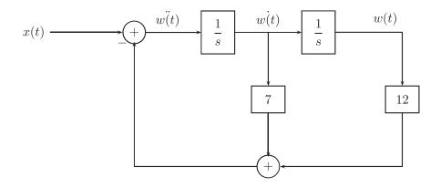
Here, note that  $\ddot{w}(t) = \frac{d^2w(t)}{dt^2}$  and  $\dot{w}(t) = \frac{dw(t)}{dt}$ . It is easy to confirm that the above implementation of the system indeed represents the system P(s) by recursively applying Black's formula.
