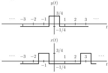
**Problem 3** Determine the Fourier series coefficients for the periodic signal x[n] depicted below. Plot the magnitude and phase of these coefficients.
