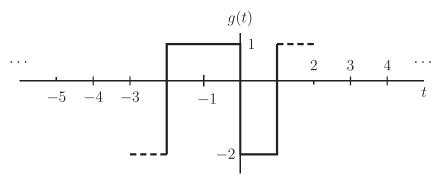
Note that g(t) must have a zero DC level, otherwise a ramping signal will be included in x(t) making it non-periodic, and unbounded. By definition, g(t) should have a zero DC level because the derivative operation eliminates it, so this can be used as a double-check.
