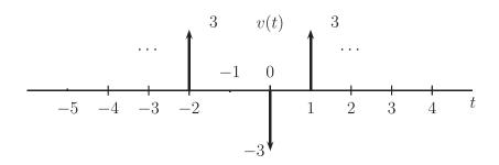
To find  $c_k$ , the Fourier series coefficients of v(t), let's take the period between -1 and 2, which contains two impulses.
