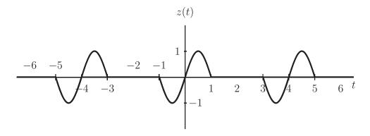
Fundamental period of z(t)=Fundamental period of  $x(t) = T = 4 \rightarrow \omega_0 = 2\pi/4 = \frac{\pi}{2}$ .
