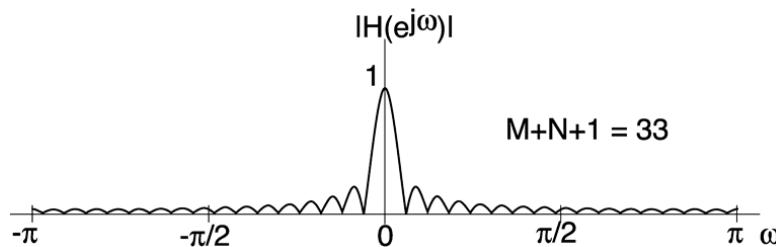
Rolls off at lower  $\omega$  as  $M+N+1$  increases
