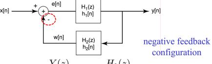
$$H(z) = \frac{Y(z)}{X(z)} = \frac{H_1(z)}{1 + H_1(z)H_2(z)}$$
