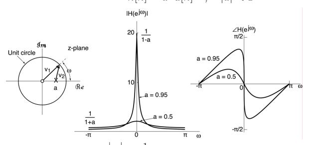
$$H(e^{j\omega}) = \frac{v_1}{v_2}, \ |H(e^{j\omega})| = \frac{|v_1|}{|v_2|} = \frac{1}{|v_2|}, \ \angle H(e^{j\omega}) = \angle v_1 - \angle v_2 = \omega - \angle v_2$$
