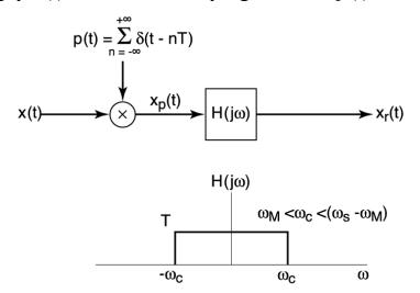
is the identity system (which is *TI*) for bandlimited x(t) satisfying the sampling theorem ( $\omega_s > 2\omega_M$ ).
