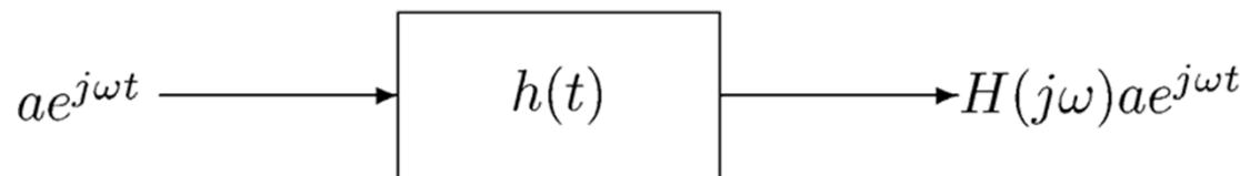
$$y(t) = \int_{-\infty}^{\infty} \underbrace{\left( H(j\omega) \frac{1}{2\pi} X(j\omega) d\omega \right)}_{H(j\omega) \cdot a} e^{j\omega t}$$
