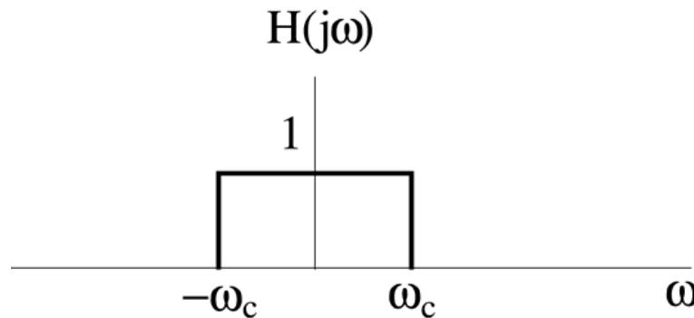
$$h(t) = \frac{1}{2\pi} \int_{-\omega_c}^{\omega_c} e^{j\omega t} d\omega$$
