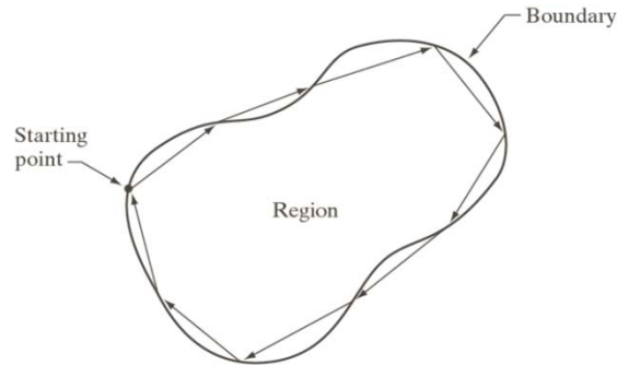
FIGURE 11.47 Coding a region boundary with directed line segments.
