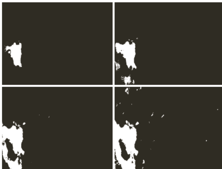
FIGURE 6.32 (a) through (d) Segmentation of Fig. 6.30(a) using option 'mahalanobis' in function colorseg with T = 25, 50, 75 , and 100, respectively. Compare with Fig. 6.31.
