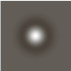
FIGURE 10.21 (a) Three-dimensional plot of the negative of the LoG. (b) Negative of the LoG displayed as an image. (c) Cross section of (a) showing zero crossings. (d) 5 \times 5 mask approximation to the shape in (a). The negative of this mask would be used in practice.
