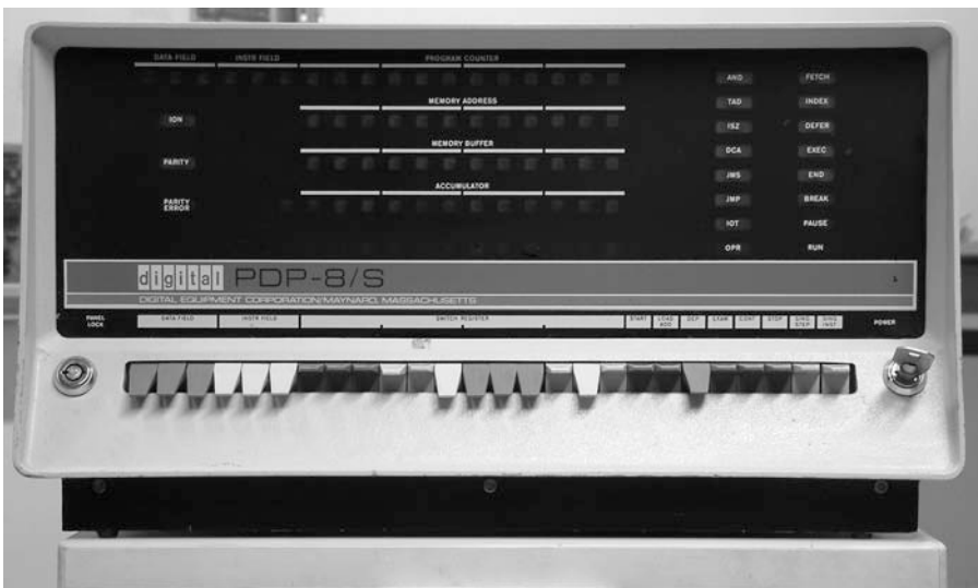
Figure 1.1: A PDP-8 computer with front panel switches for entering instructions and data. (Image courtesy of the Computer Museum at the University of Stuttgart. Photograph by Klemens Krause.)
