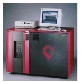
Example: Quickturn Cobalt System (1997), ~0.5M\$ for 500kgate entry level system (no photo of more recent system)
