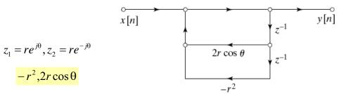
• The pole locations after quantization will be on the grid point
