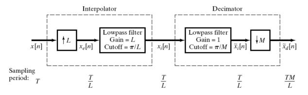
• The two low-pass filters can be combined into a single one
