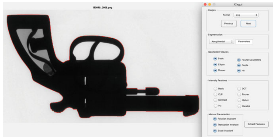
Fig. 5.28 Graphic user interface Xfxgui (see Appendix B) of XVIS Toolbox for feature extraction. In this example, all geometric features of all images of series B0049 of GDXray are extracted. In addition, the user can specify that the features to be extracted must be rotation, translation and scale invariant
