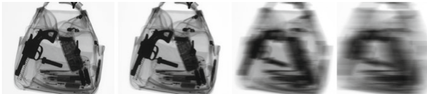
Fig. 4.33 Degradation of an X-ray image of 2208 \times 2688 pixels: Original image and degraded images with n = 32, 256 , and 512 pixels
