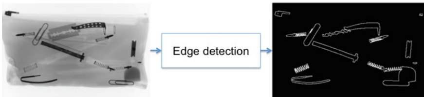
Fig. 4.15 Edge detection of an X-ray image of a pen-case. The edges correspond to the boundaries of the objects that are inside the pen-case (→ Example 4.11 📌)
