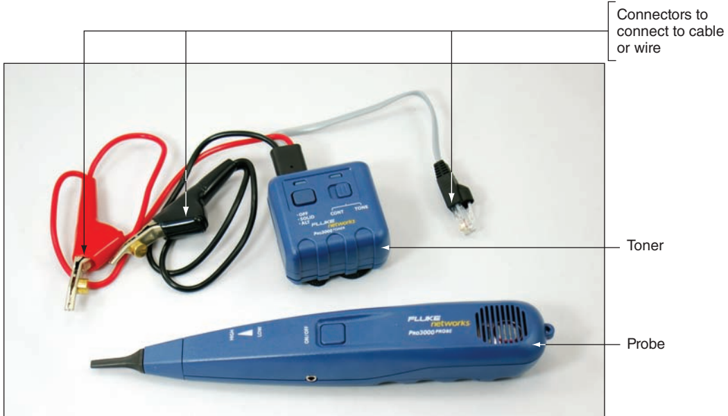
Figure 5-43 A toner and probe kit by Fluke Corporation
