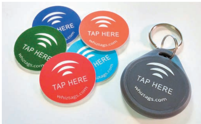
Figure 6-11 These programmable NFC tags have sticky backs for attaching to a flat surface like a wall, desk, or car dashboard
