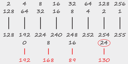
Figure 8-32 Circle the largest multiple of 8 without going over the CIDR number
