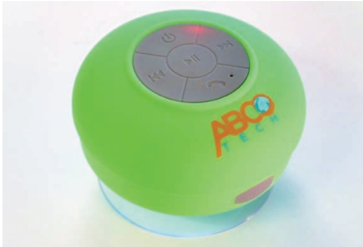
Figure 6-8 The flashing red light indicates this Bluetooth device is in discoverable mode for pairing with a smartphone or MP3 player
