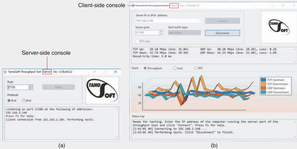
Figure 5-53 Server (a) and client (b) consoles for Throughput Test, with results showing on the client side
