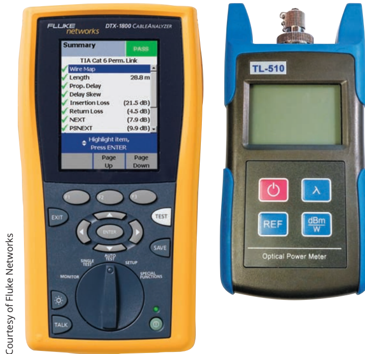
Figure 5-47 (a) On the left, the DTX-1800 device by Fluke Networks is a high-end cable performance tester designed to certify structured cabling (b) The optical power meter on the right is a more budget-friendly device that measures light power transmitted on a fiber-optic line
