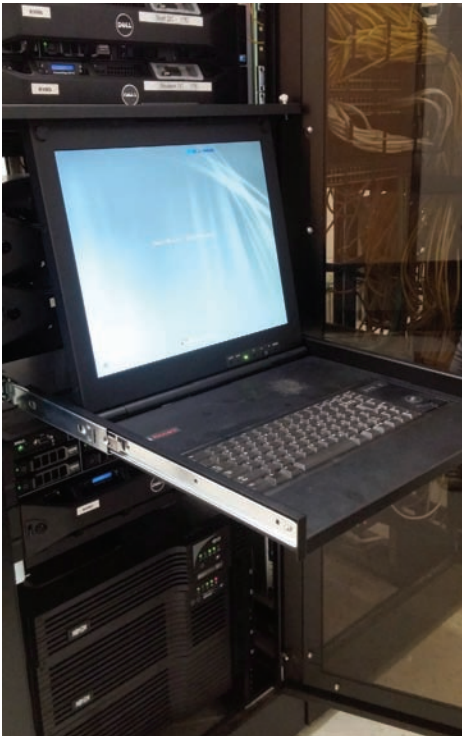
Figure 2-13 Here, a single console uses five KVM switches to access and configure multiple devices in a row of racks
