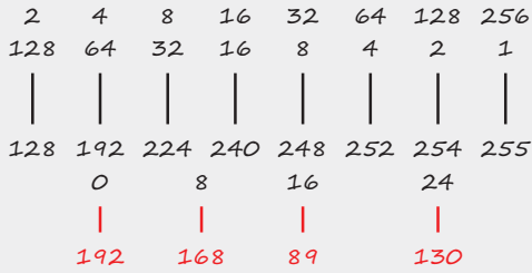
Figure 8-31 Write the host's IP address at the bottom and draw lines to connect the numbers
