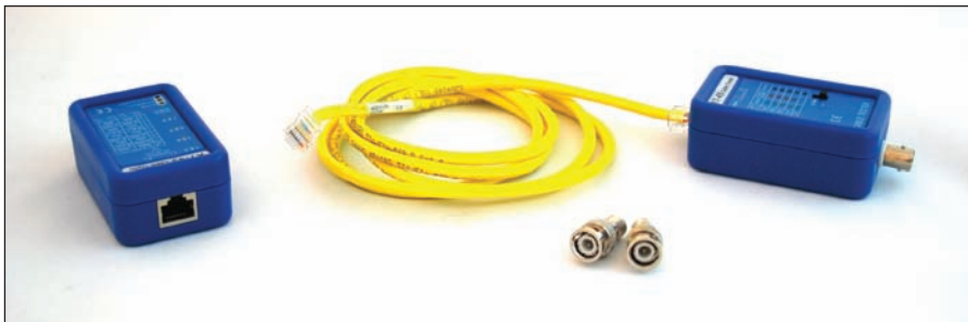
Figure 5-46 Use a cable tester pair to determine the type of cable and if the cable is good
