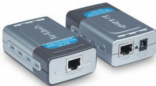
Figure 5-28 Power and data separately enter this PoE injector through ports shown on the right, and exit together through the port shown on the left
