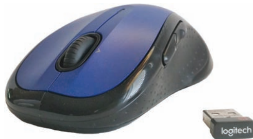
Figure 6-12 This mouse uses wireless USB to communicate with the computer and infrared to detect movement over a solid surface
