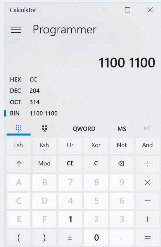
Figure 8-4 Use the Windows Calculator app to convert between decimal and binary
