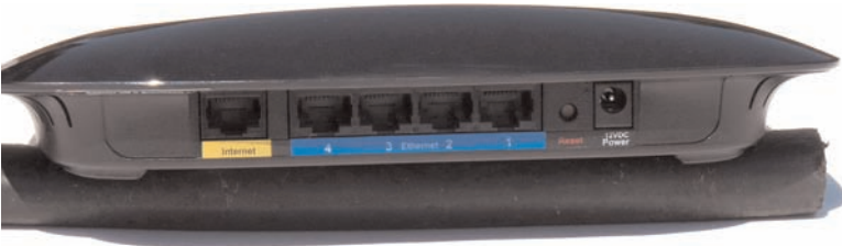
FIGURE 7.1 A wireless broadband router for a small network.
