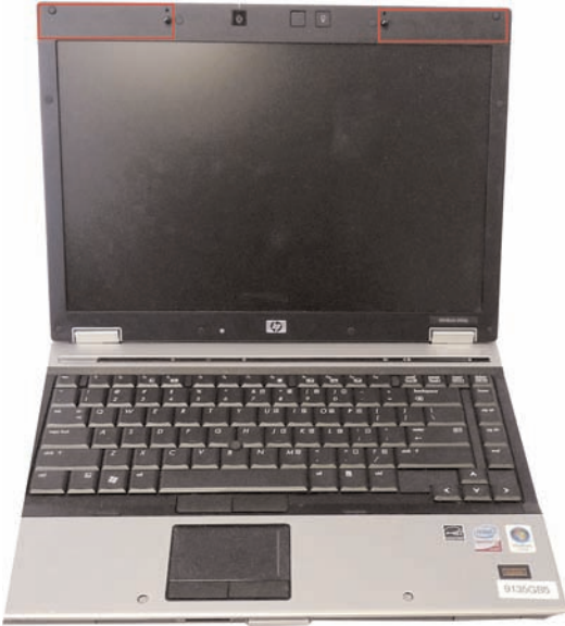
FIGURE 7.3 The antenna in a laptop is often built into the space behind the screen.
