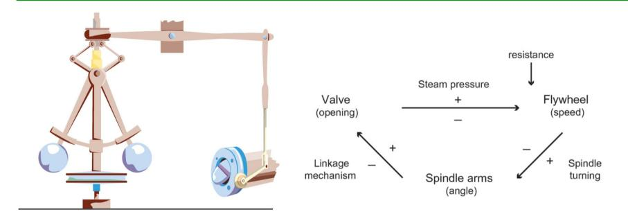
The governor regulates speed by compensating almost instantaneously when the speed of the flywheel is overshooting or undershooting.
