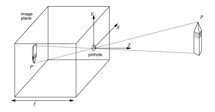
P is a point in the scene, with coordinates (X,Y,Z) P' is its image on the image plane, with coordinates (x,y,z)
