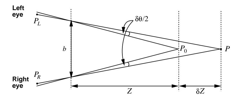
Simple geometry:  $\delta Z = Z^2 \delta \theta/(-b)$
