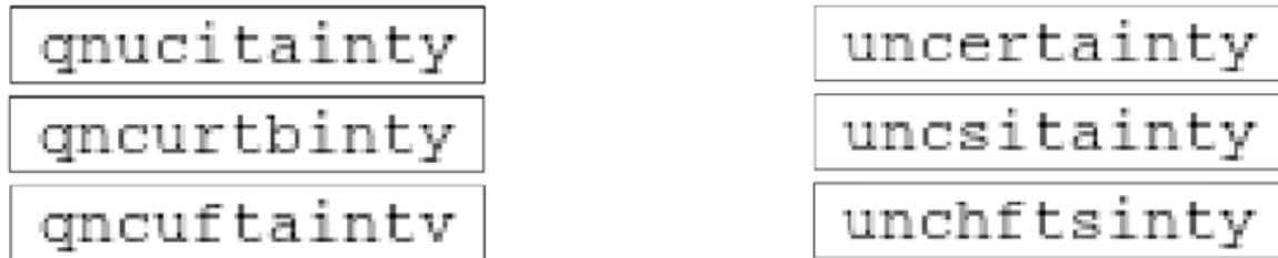
Top: extremely noisy input image. Bottom left: with three inference results from 25 MCMC iterations with the independent-letter model from Figure 15.11 . Bottom right: three inference results with the letter bigram model from Figure 15.15 . Both models exhibit ambiguity in the results, but the latter model's results reflect prior knowledge of plausible letter sequences.
